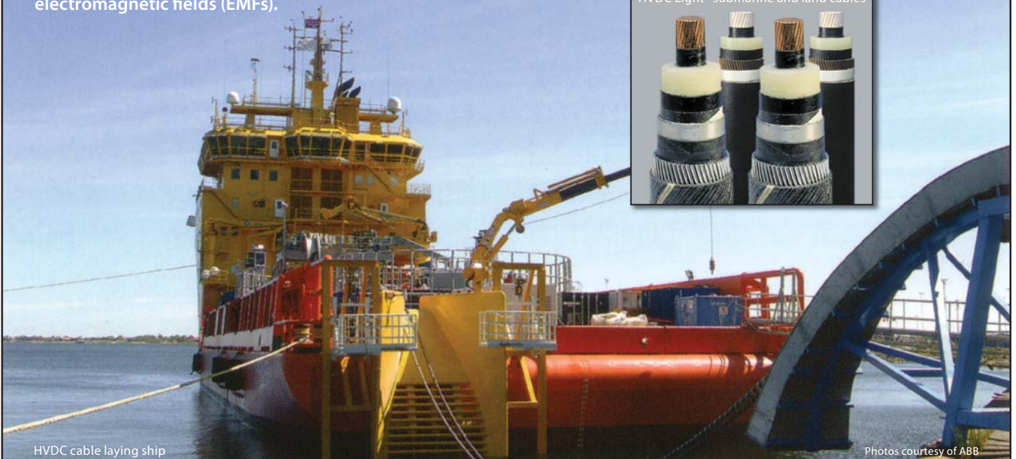
HVDC cable laying ship
